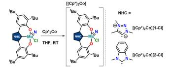
Scheme 2 Synthesis of one-electron reduced complexes [1-Cl]<sup>-</sup> and [2-Cl]<sup>-</sup> using decamethylcobaltocene as a reductant.
