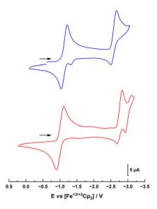
Fig. 3 Cyclic voltammograms of complexes 1-Cl (blue trace, top) and 2-Cl (red trace, bottom) in THF with 0.15 M  $NBu_4PF_6$  as a supporting electrolyte. Scan rate is shown at 100 mV s<sup>-1</sup>.
