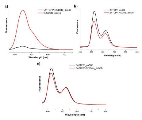
Fig. 5 Fluorescence emission spectra in DMSO solutions of (a) ZnTCPP-NCDots and NCDots upon excitation at 345 nm, (b) ZnTCPP-NCDots (concentration =  $0.003 \text{ mg mL}^{-1}$ ) and ZnTCPP (concentration =  $0.26 \times 10^{-6} \text{ M}$ ) upon excitation at 430 nm and (c) ZnTCPP-NCDots (concentration =  $0.003 \text{ mg mL}^{-1}$ ) and ZnTCPP (concentration =  $0.26 \times 10^{-6} \text{ M}$ ) upon excitation at 560 nm.
