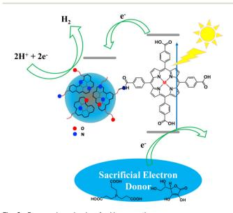
Fig. 6 Proposed mechanism for H<sub>2</sub> generation.
