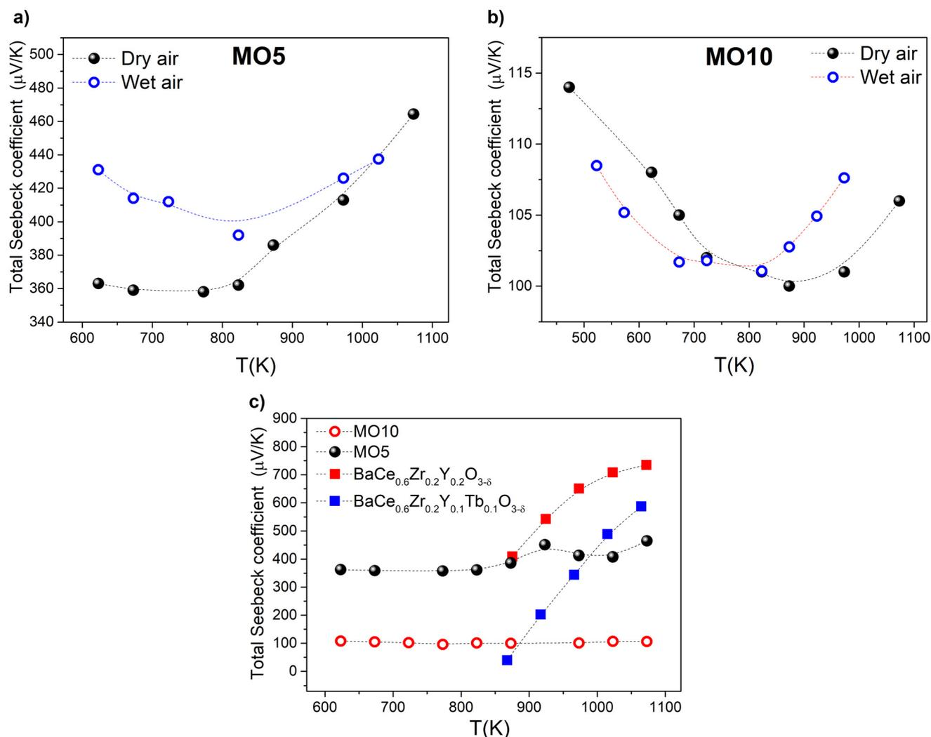
Fig. 6 Comparison of the temperature dependencies of the Seebeck coefficient for (a) MO5 and (b) MO10 samples measured in dry air as well as well-known protonic conductors – (c) BCZY and BCZY doped with terbium.
