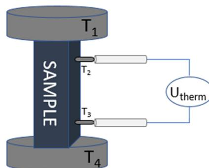
Fig. 1 Experimental scheme of Seebeck coefficient measurement.
