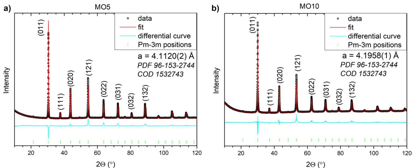
**Fig. 2** X-ray diffraction patterns with Rietveld refinement profiles and Miller indices of (a) MO5 and (b) MO10 samples.
