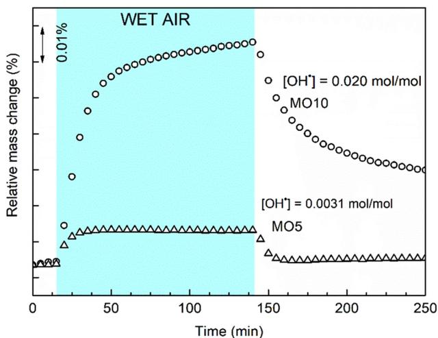
Fig. 3 Mass change of  $\text{Ba}(\text{Zr}_{0.2}\text{Hf}_{0.2}\text{Sn}_{0.2}\text{Ti}_{0.2}\text{Fe}_{0.2})\text{O}_{3-\delta}$  and  $\text{Ba}(\text{Zr}_{0.1}\text{Hf}_{0.1}\text{Sn}_{0.1}\text{Ti}_{0.1}\text{Co}_{0.1}\text{Ce}_{0.1}\text{Bi}_{0.1}\text{Fe}_{0.1}\text{Y}_{0.1}\text{Zn}_{0.1})\text{O}_{3-\delta}$  recorded after isothermal switch at 573 K between dry and humidified air.
