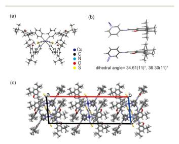
**Fig. 4** Crystal structure of **Co1**. (a) ORTEP drawing with 50% probability, (b) dihedral angles of the SAP ligands, and (c) crystal packing along the b-axis.
