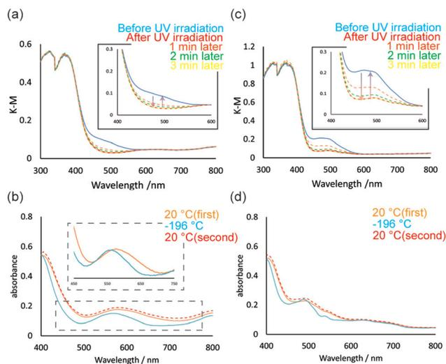
**Fig. 5** (a) and (c) UV-vis spectra of **Ni1** and **Co1** crystals before and after UV irradiation. The absorbance at 400–450 nm was increased upon UV light irradiation, and gradually decreased under visible light irradiation (550 nm). (b) and (d) UV-vis spectra of **Ni1** and **Co1** crystals for the temperature change from 20 °C to  $-196$  °C to 20 °C.
