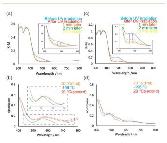
Fig. 5 (a) and (c) UV-vis spectra of Ni1 and Co1 crystals before and after UV irradiation. The absorbance at 400-450 nm was increased upon UV light irradiation, and gradually decreased under visible light irradiation (550 nm). (b) and (d) UV-vis spectra of Ni1 and Co1 crystals for the temperature change from 20 °C to -196 °C to 20 °C.
