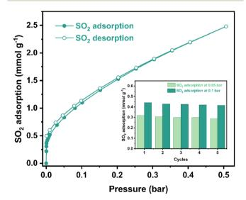
Fig. 2 Experimental SO<sub>2</sub> adsorption-desorption isotherm collected for a fully activated [NiSi]@NU-1000 sample (filled green diamonds = adsorption; open green diamonds = desorption) at 298 K and up to 0.5 bar. Inset: adsorption-desorption cycles for SO<sub>2</sub> in [NiSi]@NU-1000 at 0.05-0.1 bar and 298 K. The reactivation step was carried out only by applying vacuum (1.7  $\times$  10<sup>-3</sup> torr) for 45 minutes at room temperature (298 K).
