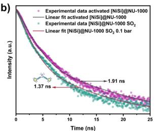
Fig. 3 (a) Solid-state emission spectra of activated [NiSi]@NU-1000 (purple line), and after exposure to 0.1 bar of SO<sub>2</sub> (green line), CO<sub>2</sub> (orange line), and air (blue line). The excitation wavelength was set at 350 nm. (b) time-resolved photoluminescence decay spectra of activated [NiSi]@NU-1000, and after exposure to 0.1 bar of SO<sub>2</sub> measured at 335.6 nm excitation and at 500 nm emission.
