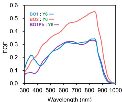
Fig. 4 EQE spectra of BO1 : Y6, BO2 : Y6, and BO1Ph : Y6 OPVs.
