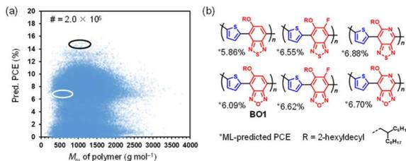
**Fig. 1** (a) Plot of ML-predicted PCE and molecular weight of the repeating unit ( $M_{ru}$ ) of the polymer. The number of these virtually generated polymers is  $\sim 200$  thousand. The area of the black ellipse is the high PCE region and that of the white ellipse is the target in this study. (b) Selected candidates of simple-structured polymers. The appended values are ML-predicted PCE. BO1 (the bottom left) was chosen as the target in this study.
