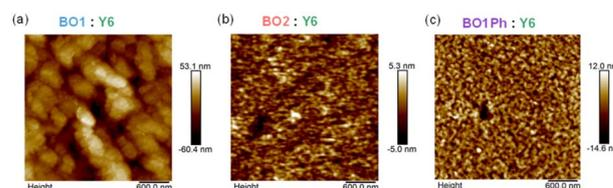
Fig. 5 AFM height images of (a) BO1 : Y6, (b) BO2 : Y6, and (c) BO1Ph : Y6 films. The scale bar is 600 nm (the size is  $2 \times 2 \mu\text{m}^2$ ). RMS values are 11.9, 1.2, and 1.5 nm for (a)–(c), respectively.
