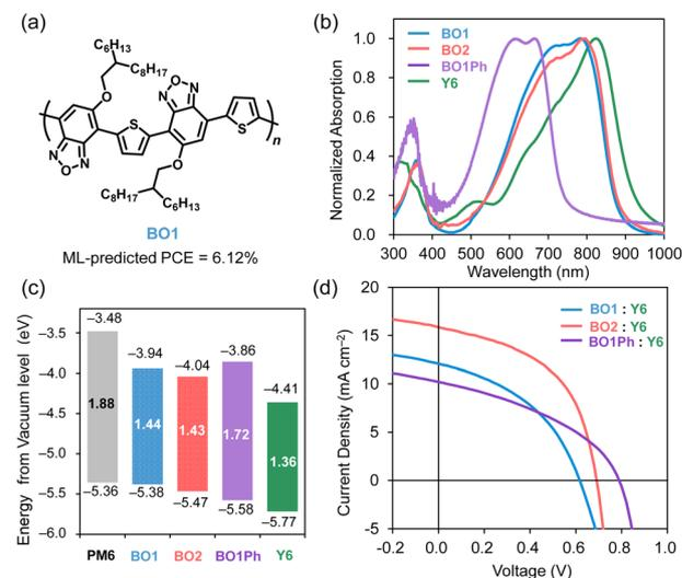
**Fig. 2** (a) Structure of the BO1 polymer that was modified from the original structure Fig. 1b because of the synthetic reason (see the main text). (b) UV-vis absorption spectra of BO1, BO2, BO1Ph (*vide infra*) and Y6 films. (c) Energy diagram of PM6, BO1, BO2, BO1Ph, and Y6; data for PM6 and Y6 were taken from the literature.<sup>45</sup> (d) JV curves of BO1:Y6, BO2:Y6, and BO1Ph:Y6 OPVs.
