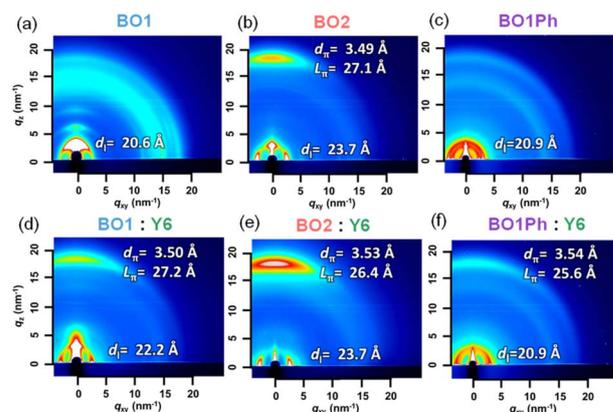
Fig. 6 2D-GIXRD images of (a) BO1, (b) BO2, (c) BO1Ph, (d) BO1 : Y6, (e) BO2 : Y6, and (f) BO1Ph : Y6 films. The calculated  $\pi$ – $\pi$  distance ( $d_{\pi}$ ), its crystallite coherence length ( $L_{\pi}$ ), and interlamellar distance ( $d_l$ ) are appended.
