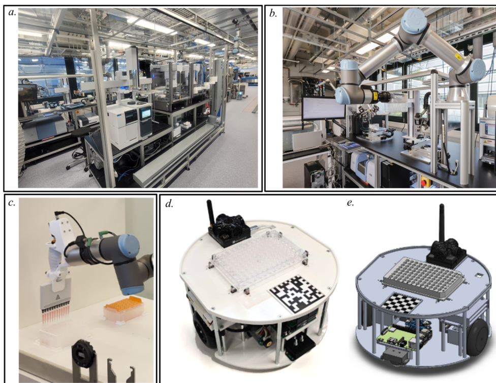
Fig. 3 (a) This is an illustration of the analytical and liquid sample preparation station, which is equipped with a six-axis Universal Robot UR3 Cobot (depicted in the upper right of the image) for the transfer of samples from the drones to the vertical storage tower. From the storage tower, a SCARA KX-2 1000 mounted on a 2.5-meter linear axis serves all the scientific equipment, including an Agilent Intuvo GC-MS equipped with PAL automation, two Agilent Bravo liquid handling stations, a microcentrifuge, a PlateLoc, and a Plate Labeler. (b) A front view of the same stations as in Fig. 2b. Here, a 6-axis UR5e is used to connect the track to an Agilent PlateLoc and to a locally developed ensemble of valves used to collect the flows from an Agilent 1290 preparative LC and distribute the samples directly to a Bruker Invenio FT-IR spectrometer, an Agilent Cary 60 UV-VIS spectrometer, and fill and seal 1.7 mm NMR rack tubes and SBS sample plates are prepared for injection into the Agilent SFC-IM-Q-TOF (6560C). This second locally developed station, derived from an Agilent RapidFire, provides internal sample transfer via microfluidics or a SCARA Precise Automation PF3400 robotic arm. (c) A development done with Techvolver. 27 The apparatus is designed to be integrated with a UR5e robot, enabling the use of manual pipettes. It is currently employed for direct sample processing and to enhance the flexibility of the stations. (d and e) Depiction of a real image and a CAD representation, respectively, of the drones utilized within the track for long-distance transfers. The drones are equipped with a wide-angle camera, which is used for locating the distributed Aruco codes. Additionally, a Datamatrix code 22,23 is employed in conjunction with the industrial cameras to inform the system of the drone's identity and its precise alignment with respect to the 6-axis cobot and the SBS format sample plate. 28
