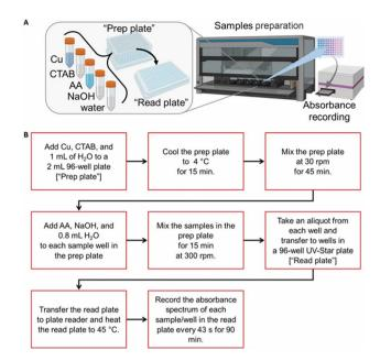
Fig. 1 Experimental robotic synthesis of the copper nanoclusters (A). Experimental setup and (B). Schematic for dispensing the reagents at various molar concentration (see SI Table 1) and subsequent absorbance measurement of CuNCs.
