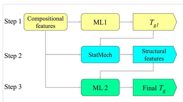
Fig. 7 Three-step workflow for improved  $T_g$  predictions.
