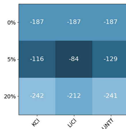
Fig. 9 Heat map of the variation in reaction rate with salt additives shows a non-linear relationship with small quantities decreasing degradation while larger quantities promote it.
