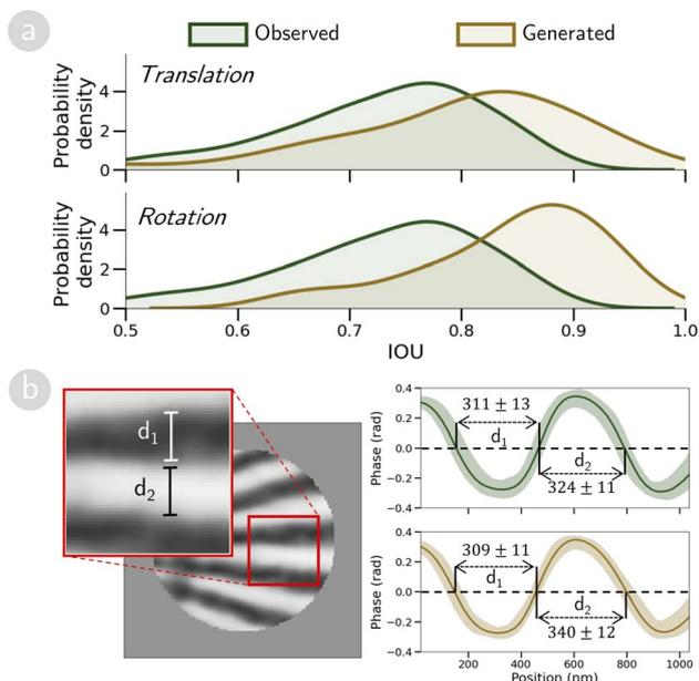
Fig. 4 Proof-of-concept validation of generative modeling on motions of Ta test chart. (a) Intersection-over-union (IOU) distributions between consecutive frames for translation and rotation sequences, comparing observed (green) and generated (yellow) data. (b) Comparison of slit widths extracted from observed and generated CXDI images, where solid lines represent average slit width in the matched region, and the spectrum illustrates width fluctuations.
