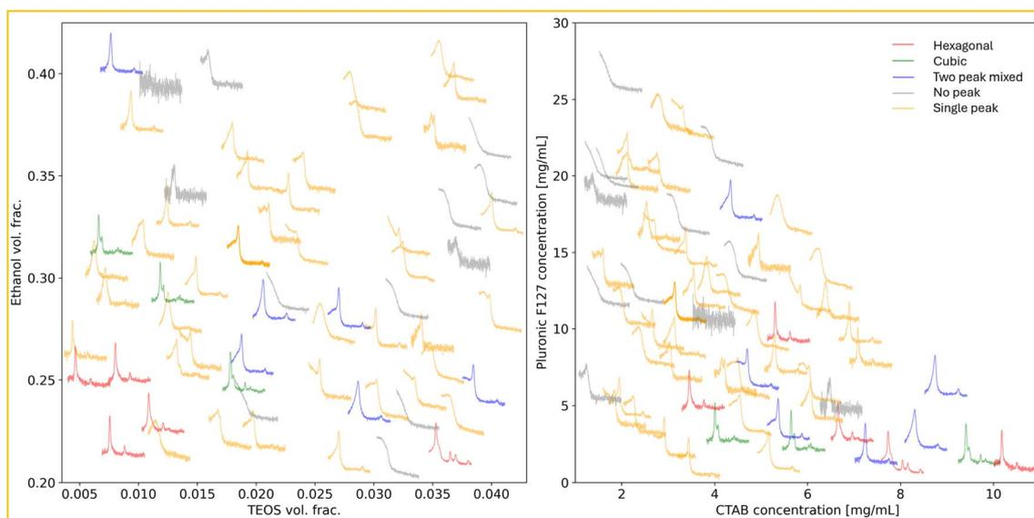
Fig. 7 Composition-scattering plots for SAXS measurements of samples. This plot is analogous to Fig. 5 but shows high- $Q$  scattering associated with porous phase order from the same samples. Individual sample scattering is colored according to the identified internal pore phase.
