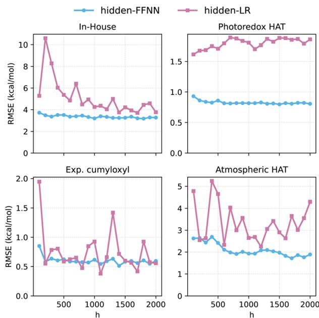
**Fig. 3** Test RMSE of models based on hidden space with varying hidden sizes  $h$  (surrogate model trained with the full set of descriptors) for a selection of downstream datasets. The performance of FFNNs is compared to that of LR models.
