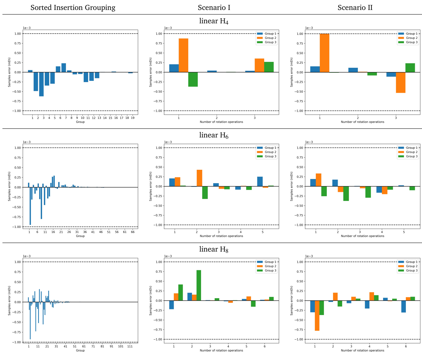
Fig. 4 Finite samples simulation for three molecules: linear H_4 , linear H_6 , linear H_8 . SI method is used as a benchmark. In Scenario I and II, the rotation operations and the measured groups correspond to those used for the approximation of Hamiltonian expectation values. As mentioned above we set a threshold precision of \varepsilon = 10^{-3} .
