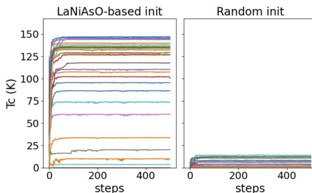
Fig. 3 Comparison of optimisation results under different initialisation methods. Both approaches employ Adam optimiser<sup>40</sup> with a learning rate of 0.001. (Left) Initialisation by adding noise to an existing superconductor (LaNiAsO). (Right) Random initialisation, in which seven elements are chosen arbitrarily and assigned random compositional values.
