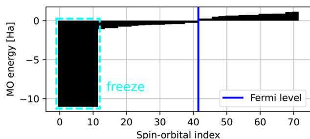
Fig. 3 Benzene ( $\text{C}_6\text{H}_6$ ) STO-3G molecular orbital energies computed with the restricted Hartree–Fock method. The lowest twelve spin-orbitals may be frozen without dramatically affecting ground-state energy estimates.
