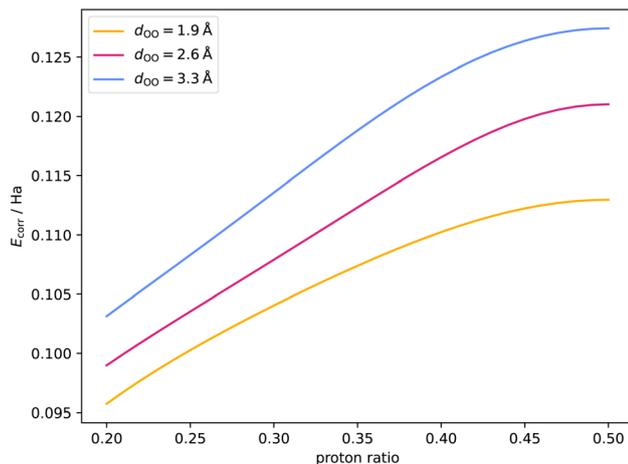
Fig. 8 The correlation energy  $E_{\text{corr}} = E_{\text{HF}} - E_{\text{FCI}}$ , as a function of proton ratio  $r$ . Restricted-HF and full-CI calculations are performed on a single Zundel cation (the atoms in blue region of Fig. 7) at three water separation distances with the STO-3G basis set. Across the three water separations, the mean correlation energy increase from  $r = 0.2$  to  $0.5$  is 21%.
