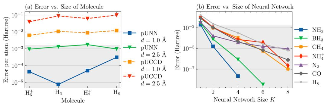
Fig. 4 Factors for the accuracy of the pUNN method. (a) The error of pUNN versus the size of the molecule under study. (b) The error of pUNN versus the size of the neural network  $K$ . The number of hidden neurons in the neural network is  $2KN$  where  $N$  is the number of molecular orbitals. The shaded area indicates the chemical accuracy.
