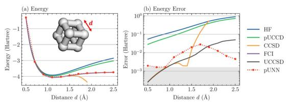
Fig. 5 Benchmarking pUNN based on the potential energy profile of cubic  $H_8$ . (a) The potential energy profile of cubic  $H_8$  by different computational methods. (b) The error compared with the exact solution *versus* the H–H distance in the  $H_8$  cube.
