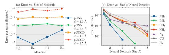
Fig. 4 Factors for the accuracy of the pUNN method. (a) The error of pUNN versus the size of the molecule under study. (b) The error of pUNN versus the size of the neural network K. The number of hidden neurons in the neural network is 2KN where N is the number of molecular orbitals. The shaded area indicates the chemical accuracy.
