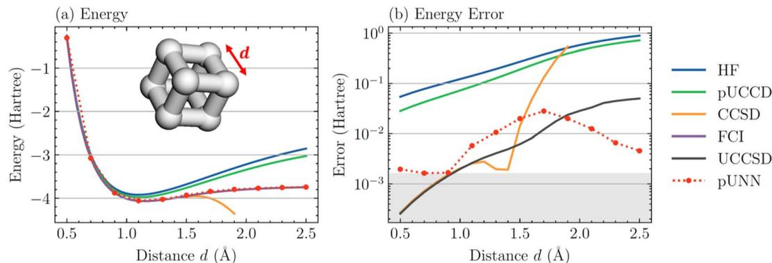
Fig. 5 Benchmarking pUNN based on the potential energy profile of cubic  $H_8$ . (a) The potential energy profile of cubic  $H_8$  by different computational methods. (b) The error compared with the exact solution versus the H–H distance in the  $H_8$  cube.
