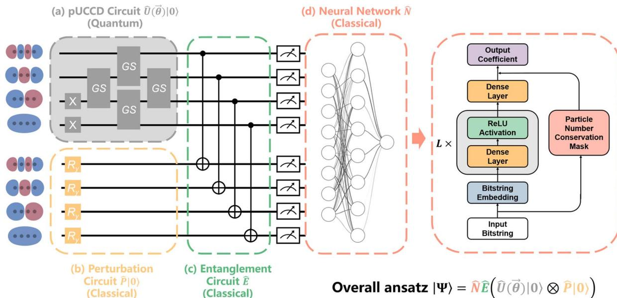
**Fig. 1** A schematic diagram for the pUNN framework. The (a) pUCCD circuit in the grey box is the only component executed on a real quantum computer. "GS" denotes Givens–Swap gate. Meanwhile, the (b) perturbation circuit and the (c) entanglement circuit are processed classically. Together, the quantum circuit and the (d) neural network serves as an ansatz and are trained jointly to represent the molecular wavefunction.
