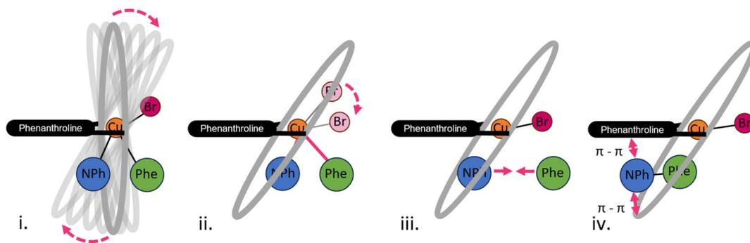
Fig. 9 Schematic representation of the movements corresponding to the reaction coordinate of the C–N coupling reaction. (i) Tilting movement of the calixarene cage; (ii) Change in coordination of the copper centre; (iii) Shortening of the C–N bond; (iv)  $\pi$ - $\pi$  stacking effects stabilise the product in the cavity.
