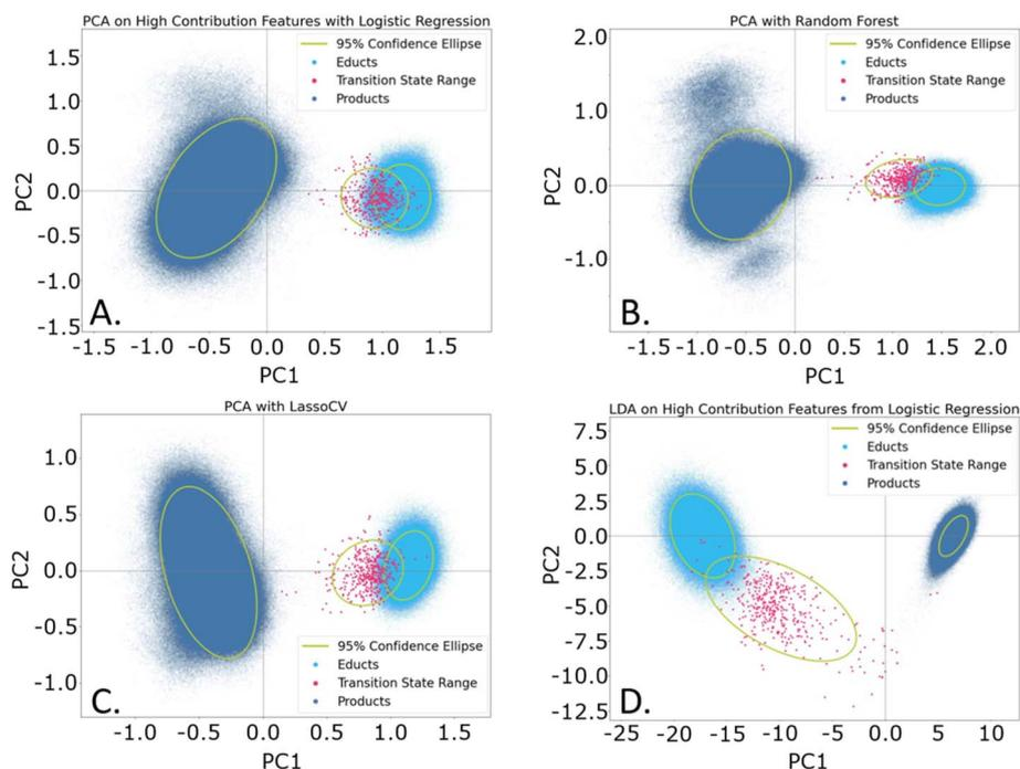
Fig. 3 Dimensionality reduction performance with various feature reduction methods: (A). PCA with Logistic Regression with mean-based cutoff; (B). PCA with Random Forest with mean-based cutoff; (C). PCA with LassoCV; (D). LDA with Recursive Feature Elimination with cross validation using a Logistic Regression classifier.
