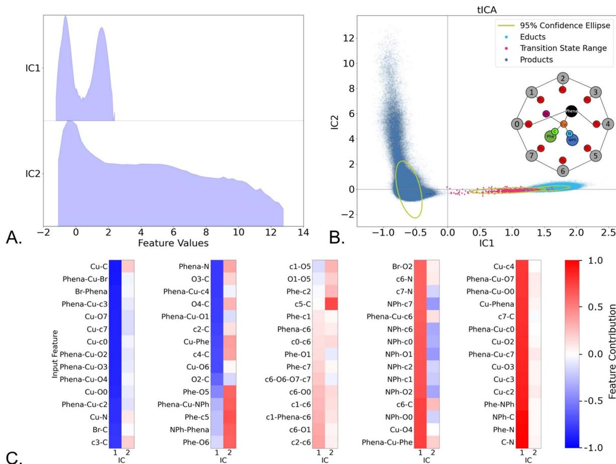
Fig. 5 Time-lagged independent component analysis of the MD trajectories, using a lag time of 20 fs. (A) Distribution of the structural ensembles (feature values) over the first two independent components; (B). Projection of the ensembles in the space of independent components 1 and 2 (IC1 and IC2), with the ensemble colouring performed *a posteriori*; (C). Normalized internal coordinate (feature) contribution to each independent component.
