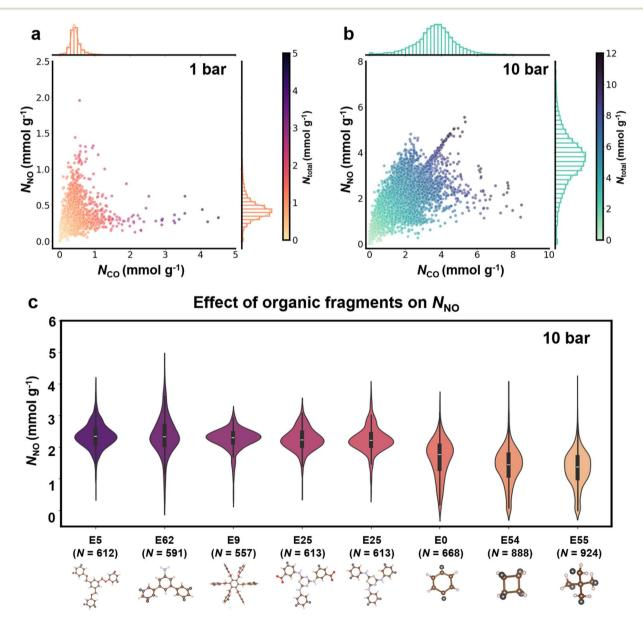
Fig. 3 Relationships between  $N_{NO}$  and  $N_{CO}$  in an equimolar NO/CO mixture at 298 K under pressures of (a) 1 bar and (b) 10 bar. (c) Violin plot for the effect of common organic fragments on  $N_{NO}$  at 10 bar. The violins are sorted from left to right based on descending median  $N_{NO}$ ; see the corresponding plot for  $N_{CO}$  in Fig. S9.
