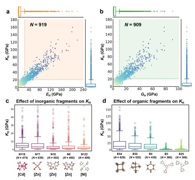
Fig. 4 (a) Bulk moduli  $K_H$  against shear moduli  $G_H$  (b)  $K_H$  against Young's moduli  $E_H$  for 10 748 Bio-hMOFs. The shaded region denotes exceptionally high moduli (1.5  $\times$  the upper threshold of the Inter-Quantile Range).  $K_H$  in Bio-hMOFs with the most common (c) inorganic fragments and (d) organic fragments, sorted by descending median  $K_H$  from left to right.
