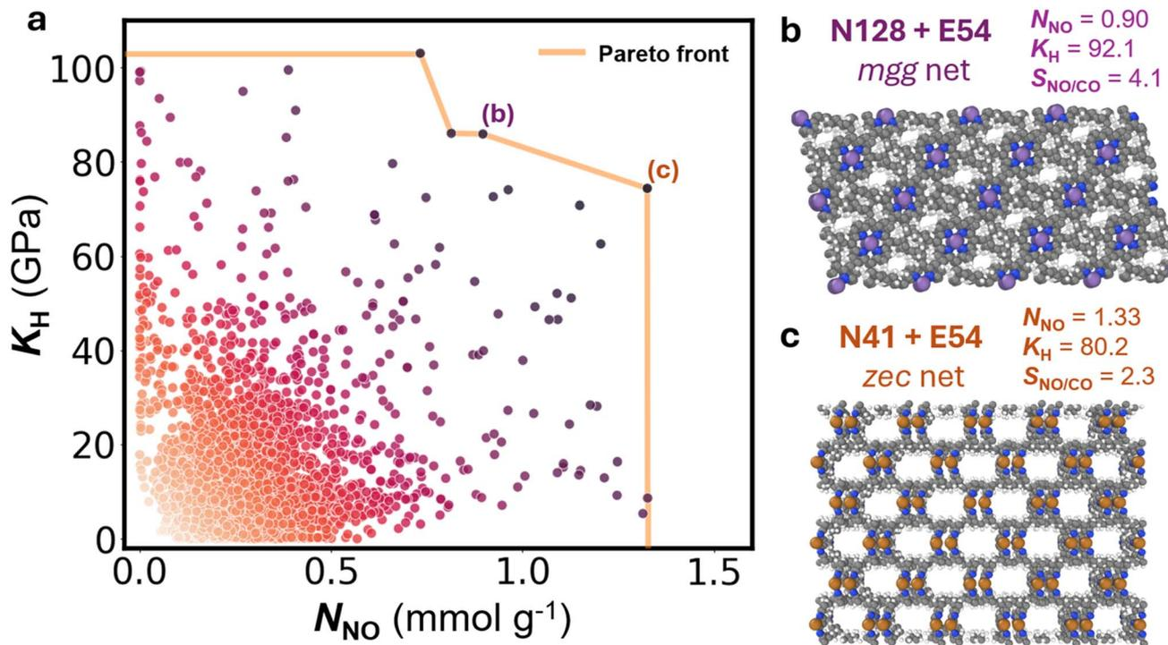
Fig. 5 (a) Relationship between  $K_H$  and  $N_{NO}$  and the Pareto frontier. (b) and (c) Structures with their fragments and topological nets. Color code: Mn (purple), Fe (bronze), N (blue), C (grey), and H (white).
