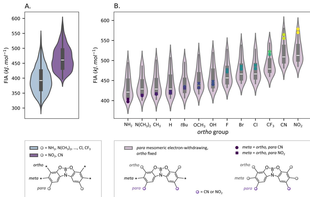
**Fig. 7** (A) Violin plots separating data between molecules possessing mesomeric electron-withdrawing groups (CN or  $\text{NO}_2$ ) in *para* position or not. (B) Distributions of molecules with a mesomeric electron-withdrawing group in *para*, separated by the *ortho* group and highlighting variations in the *meta* group; dotted markers indicate molecules where the *meta* group matches the *ortho* group.
