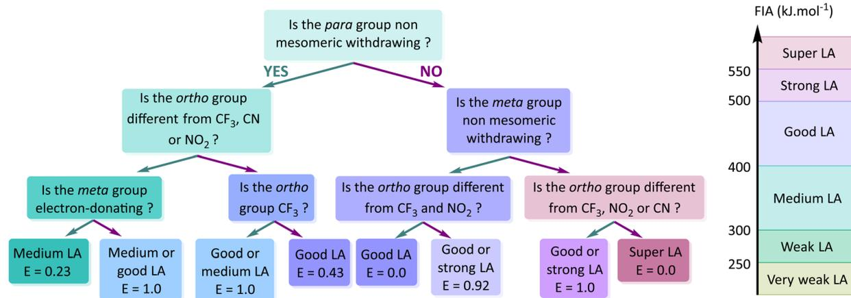
**Scheme 1** Decision tree model for the ONO structure (0.73 accuracy on 10-fold CV). Nodes are split based on Hammett-extended feature thresholds. A left arrow indicates a “Yes” decision, while a right arrow indicates a “No” decision. The entropy ( $E$ ) of each node reflects its purity, indicating whether it contains a unique class ( $E = 0$ ) or not. Original tree from Scikit-learn<sup>63</sup> is provided in Fig. S20.
