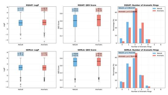
Fig. 5 Comparative property distributions (log P, QED score, and aromatic ring counts) for molecules generated by EQGAT and SemlaFlow models trained on kekulized versus explicit-aromatic GEOM-drugs datasets. No significant shifts are observed across these properties, indicating that kekulization does not introduce bias in the learned chemical space representation.
