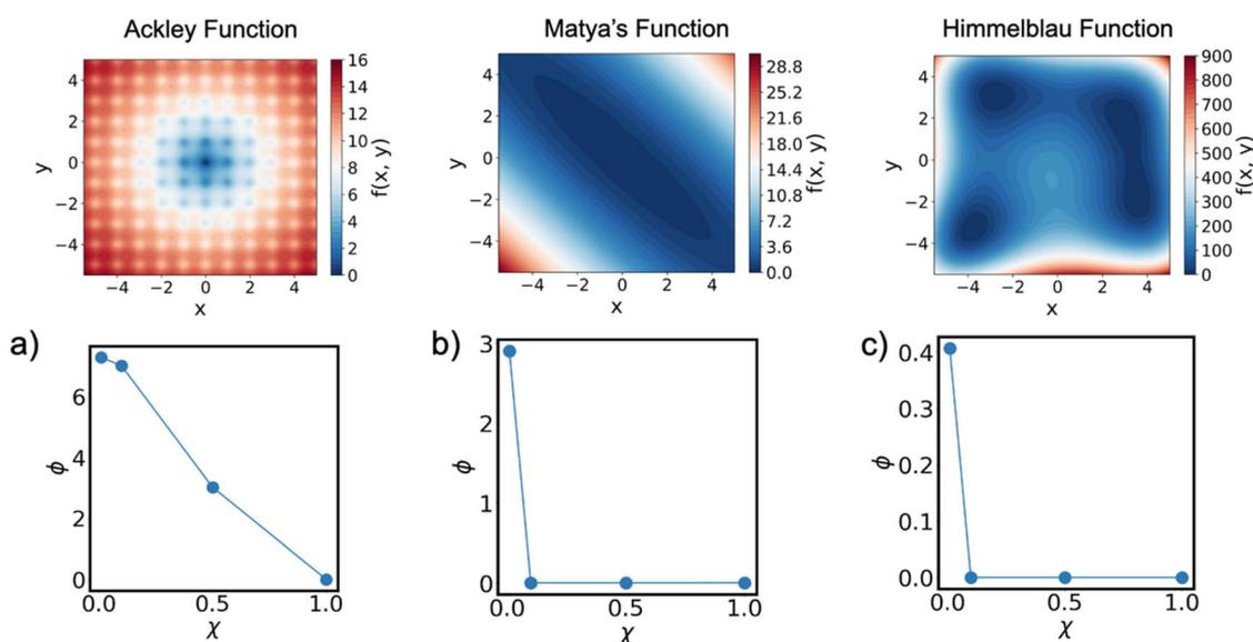
Fig. 3 Visual maps of the three investigated functions – Ackley, Matyas, and Himmelblau – depicting the distribution of minima and maxima across the input space. The plots below illustrate  $\phi$  convergence for the respective functions: (a) Ackley, (b) Matyas, and (c) Himmelblau.
