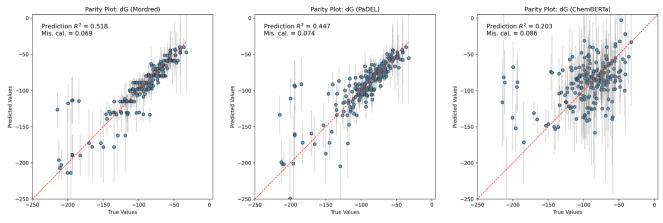
Fig. 7 Prediction performance for  $\Delta G_{\text{solv}}$  using MolDAIS-MI (K=5) for the various descriptor libraries. Left to right: Mordred, PaDEL, Chem-BERTa. Each plot shows the parity between predicted and ground truth values on the test set.  $R^2$  values (higher is better) and miscalibration areas (lower is better) are also reported in the top left corner of each plot.
