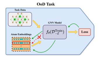
Fig. 1 Since OoD elements are absent from the training dataset, their corresponding embedding vectors receive no backpropagated gradients and thus remain static throughout the optimization process.
