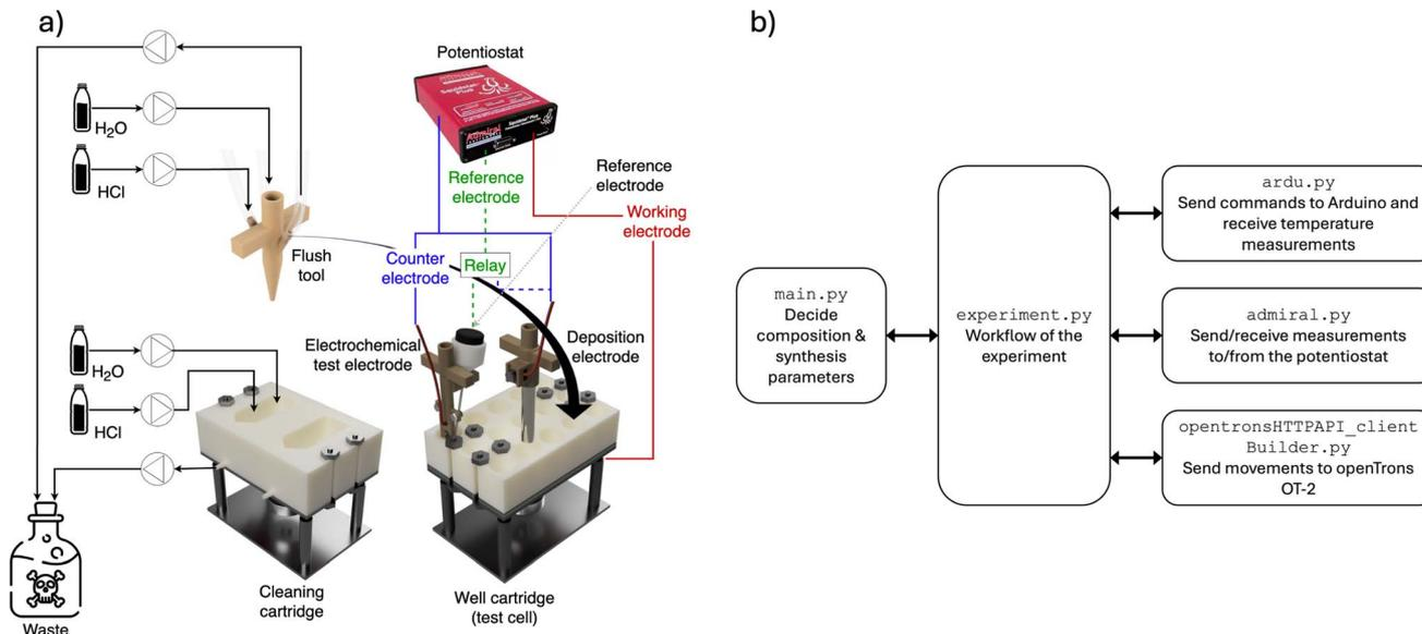
Fig. 3 (a) Schematic of the AMPERE-2 electrodeposition setup, showing the connection between the potentiostat, pumps, and functional tools. (b) Overview of software structure: *main.py* initializes the workflow by setting experimental parameters such as temperature, deposition current, and metal precursor combinations. These parameters are passed to *experiment.py*, which coordinates control of Arduino, potentiostat, and OT-2.
