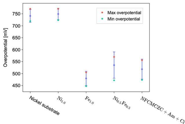
Fig. 8 Reproducibility of OER measurements across replicate catalyst samples, assessed by the variation in potential at  $50 \text{ mA cm}^{-2}$ . The blue dots represent the mean overpotential, error bars indicate the standard deviation, and the red and green markers denote the maximum and minimum values observed within each sample set.
