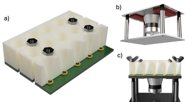
**Fig. 2** (a) Cross-sectional view of the array reactor, displaying the cone-shaped wells and nickel foil (green) functioning as the working electrode, separated by a yellow silicone O-ring to ensure a sealed interface. (b) Base cartridge equipped with ultrasound, heating elements, and rubber dampeners for vibration absorption. (c) Side view of the array reactor mounted onto the base cartridge, which also supports the mounting of the cleaning bath.
