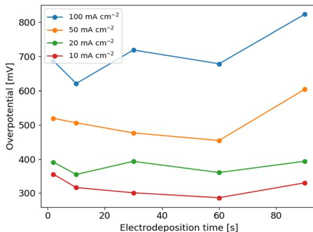
**Fig. 6** Average OER overpotential at 10, 20, 50 and  $100 \text{ mA cm}^{-2}$ , measured on NFCMCZC + Am + Ci samples electrodeposited for different durations. Values reflect the final 20 seconds of each constant current step, corrected for 90% ohmic resistance.
