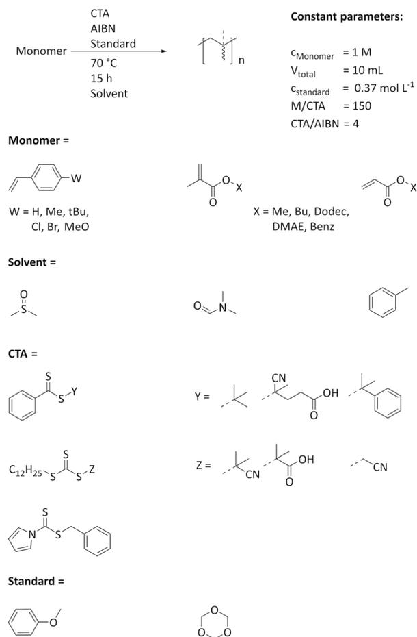
Fig. 1 Schematic representation of the performed reactions with constant parameters and variables (monomer, solvent, and CTA).
