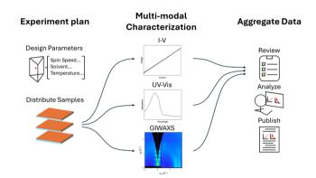
Fig. 6 SEARS: multi-facility, multi-modal data aggregation.
