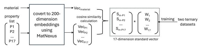
Fig. 1 Illustration plot of standard vector method.
