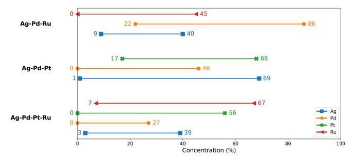
Fig. 3 Compositional ranges of synthesised materials.
