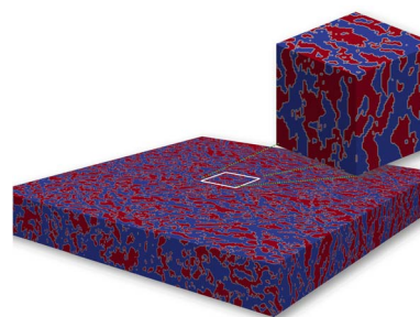
Fig. 9 Visualization of spin-cast P3HT:PCBM thin film, fabricated using chlorobenzene reconstructed using tomographic energy-filtered TEM. The main image shows the reconstructed 3D morphology, with blue and red domains representing the electron-donating (donor) and electron-accepting (acceptor) materials, respectively. The inset provides a zoomed-in view of a cubic subvolume extracted from the full morphology.
