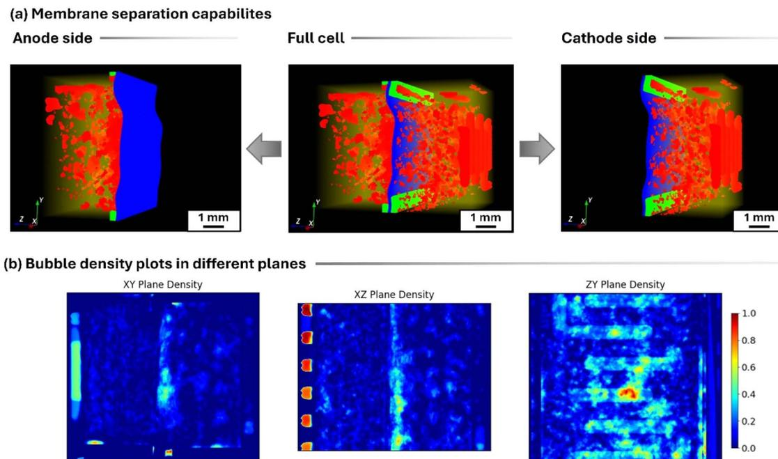
Fig. 5 (a) Showcase of the precise electrode differentiation by the software. (b) Density maps depicting the bubble spatial distribution along the cell from three different planes  $XY$ ,  $XZ$ , and  $ZY$ . Areas with warmer hues represent high bubble density, while colder colors suggest less populated zones.
