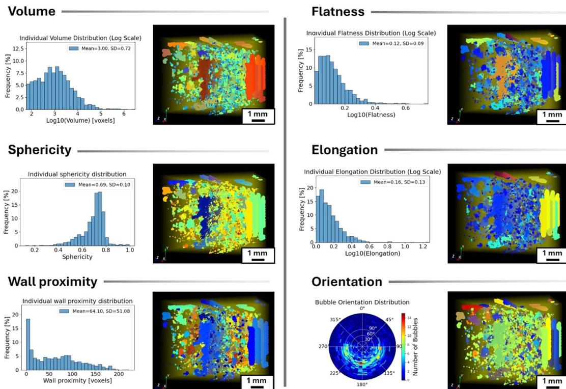
**Fig. 6** Analysis of individual bubble shape characteristics within segmented volumes. For each assessed morphological property, distribution histograms are plotted to detail the variance of properties across bubbles. Simultaneously, software-generated, color-mapped 3D visualizations represent these individual properties, where warmer colors indicate higher property values and cooler hues signify lower values.
