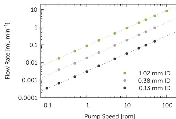
**Fig. 7** Measured flow rate of the pump across different rotation speed and sizes of peristaltic tubes. The dashed lines represent linear functions without vertical offset, that were fitted to the measurements.
