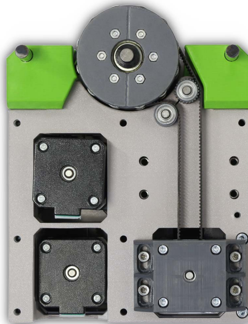
Fig. 2 Photo of the pump with the outer part of the main body and the electronic compartment removed to show the internal alignment of the motors, belt and idlers.
