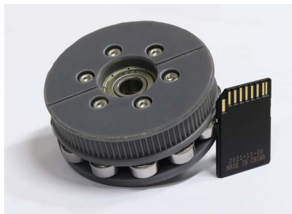
Fig. 3 Close-up picture of a rotor with the bearing rollers at the bottom and the pulley at the top. The SD card is intended to provide a sense of scale.
