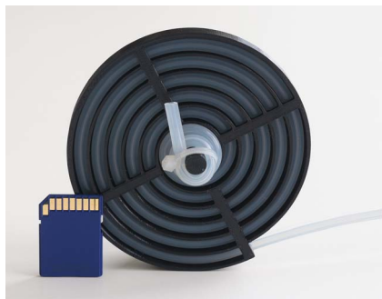
Fig. 6 Photo of the spiral reservoir. The changing weight of this reservoir is tracked during the gravimetric measurements. The SD card is intended to provide a sense of scale.
