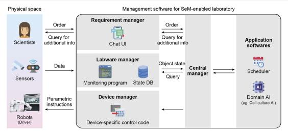
Fig. 5 An example architecture of management software for SeM-enabled laboratory. A laboratory with SeM is referred to as a SeM-enabled laboratory. The system is composed of the Central manager and three key modules: the Requirement manager, the Device manager, and the Labware manager.
