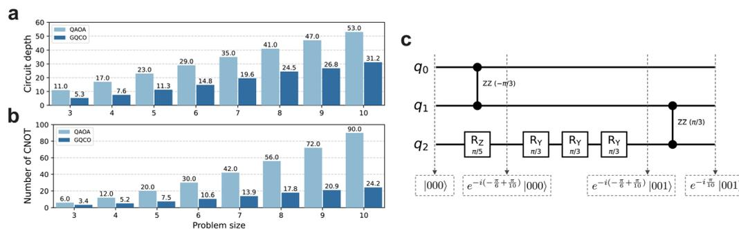
**Fig. 6** Analyses of the generated circuits. (a) Comparison of circuit depth and (b) number of CNOT gates between GQCO-generated and one-layer QAOA circuits for each problem size. (c) A representative example of a generated circuit. Six quantum gates are applied sequentially to the initial state  $|000\rangle$  to obtain the final quantum state  $e^{-i\frac{\pi}{10}}|001\rangle$ . The quantum states at two intermediate steps are also illustrated.
