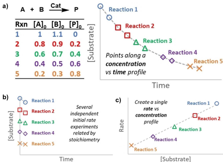
Fig. 18 Relationship between independent initial rate experiments and a single kinetic profile through SPKA. Each colour represents a new reaction, a simulated point on a single kinetic profile collecting in either batch or flow: (a) concentration vs. time plot for one experiment monitored over time; (b) concentration vs. time plot for multiple independent reactions; (c) multiple reactions creating a single SPKA kinetic profile in a rate vs. concentration plot. Reproduced with permission under the Creative Commons Attribution license (CC-BY). Copyright © 2023 Lennon and Dingwell, 138 Angewandte Chemie International Edition published by Wiley-VCH GmbH.
