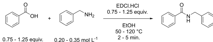
Scheme 4 Amide coupling of benzoic acid and benzylamine with EDCI·HCl ( N -(3-dimethylaminopropyl)- N' -ethylcarbodiimide hydrochloride) and EtOH (ethanol), featuring input parameter boundaries. Adapted from Wagner et al. 95 with permission under the Creative Commons Attribution license (CC-BY 4.0). Copyright © 2024, Wagner et al.
