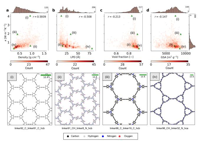
Fig. 2 Distribution of (a)  $\kappa$  versus density (with the color indicating data count per bin), (b)  $\kappa$  versus largest pore diameter (LPD), (c)  $\kappa$  versus void fraction, and (d)  $\kappa$  versus gravimetric surface area (GSA). Also shown are four COF structures (i–iv) with contrasting properties, marked by green triangles in the plots above. The r-value indicates the Pearson correlation coefficient.
