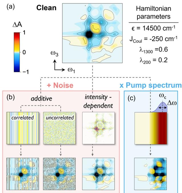
**Fig. 3** (a) A representative “clean” spectrum generated with the parameters provided in the inset table. We polluted the datasets by (b) adding one of three types of experimental noise or (c) convoluting the 2DES signal with a Gaussian pump pulse. Representative images of the isolated data pollutants are shown in the upper panels of (b) and (c); the lower panels of (b) and (c) show the resulting polluted spectra. All spectra and noise profiles are plotted against the color scale in (a).
