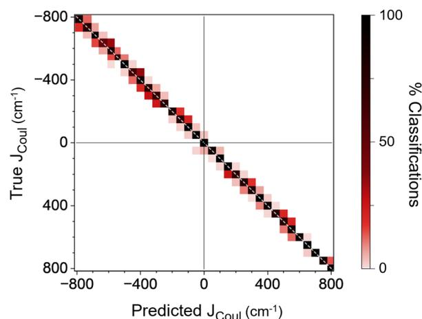
Fig. 4 Confusion matrix comparing the true vs. NN-predicted values of  $J_{\text{Coul}}$  when trained and tested on clean data. Each row is normalized to unity. Diagonal entries, indicated by the dotted white line, reflect correct classifications; off-diagonal entries report on misclassifications.
