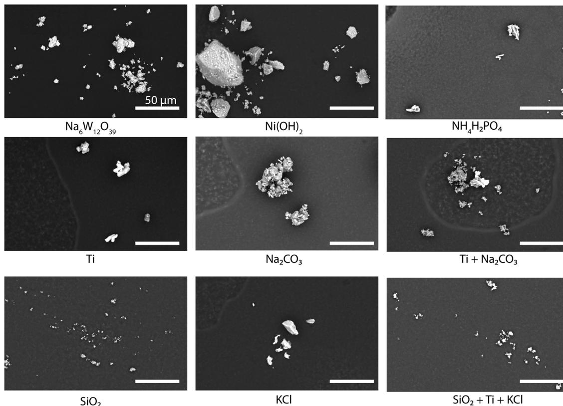
Fig. 6 SEM micrographs of various chemical compounds and powder mixtures prepared using the EMSBot. The white bar denotes a scale of 50  $\mu\text{m}$ .
