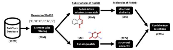
Fig. 2 Screening of organic electroactive molecules from the PubChem database based on their similarity to molecules in the reference database, RedDB.
