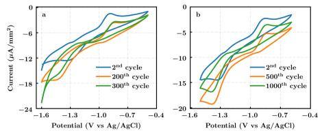
Fig. 5 Electrochemical characterization of two selected organic molecules. (a) Cyclic voltammogram of 1 mM (2-aminoethyl)[(pyrazin-2-yl) methyl]amine in 1 M KCl aqueous solution. (b) Cyclic voltammogram of N-[(pyrazin-2-yl)methyl]formamide under the same conditions. Both voltammograms were recorded at a scan rate of 20 mV s $^{-1}$ .
