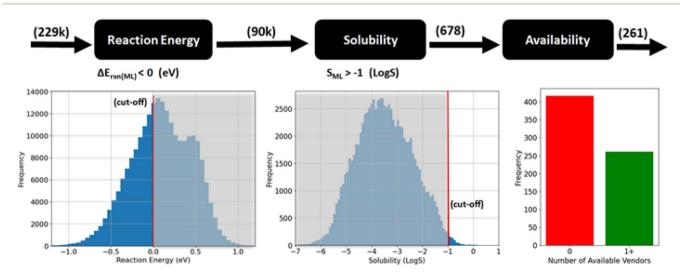
Fig. 3 Selection of molecules based on predicted properties and vendor availability. Reaction energy and solubility were predicted using the RedPred and AqSolPred ML models, respectively. Shaded areas in the histograms indicate molecules excluded due to the applied cut-off for ML-predicted properties. The bar chart illustrates the proportion of molecules that are either unavailable or available with pricing information from vendors.
