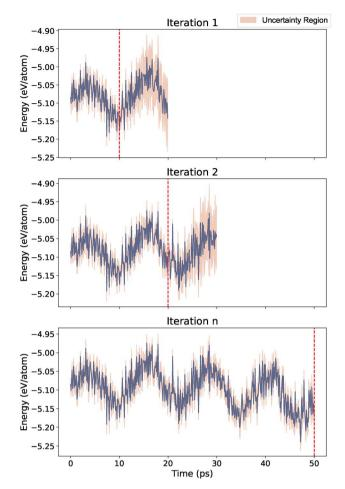
Fig. 6 Example of active learning for energy evolution over time for different iterations. The orange region indicates uncertainty. In Iteration 1 and Iteration 2, uncertainty increases significantly after the red dashed line leading to termination of the simulation. The last iteration (Iteration n) represents the case where the previous active learning iteration result in a stable, accurate, and precise simulation.
