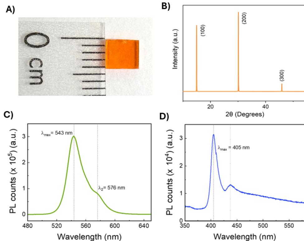
Fig. 4 (A) Image of a seedless synthesised MAPbBr<sub>3</sub> single crystal. (B) X-ray diffraction spectra of the seedless-grown MAPbBr<sub>3</sub> crystal. (C) and (D) X-ray diffraction spectra of the seedless-grown MAPbBr<sub>3</sub> crystal. (D) Photoluminescence measurements of a seed containing MAPbCl<sub>3</sub> single crystal.
