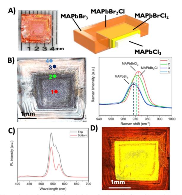
Fig. 5 (A) Picture of a mixed halides perovskite single crystal and diagram of crystal composition (B) Raman shift spectra of selected points. (C) Photoluminescence of crystal faces (D) confocal photoluminescence microscope picture of the mixed composition perovskite single crystal.
