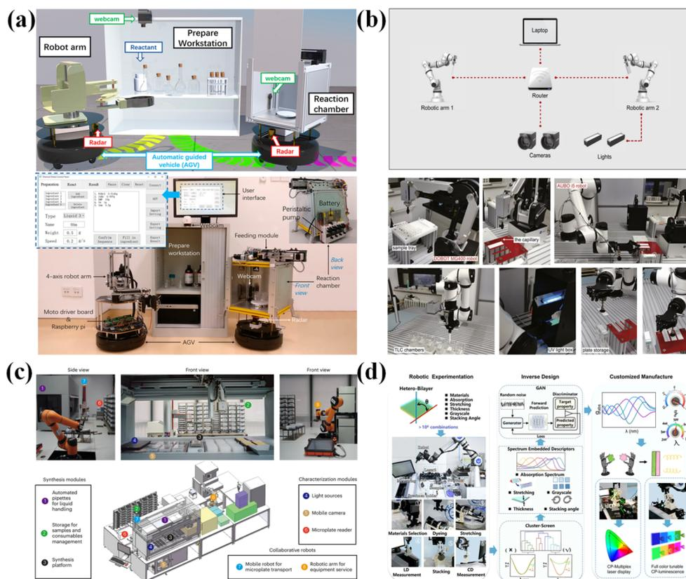
Fig. 2 Some autonomous platforms driven by iterative algorithms. (a) AIR-Chem. (b) High-throughput thin-layer chromatography. (c) Automated synthesis and *in situ* characterization platform of colloidal nanocrystals. (d) AI-Chemist.
