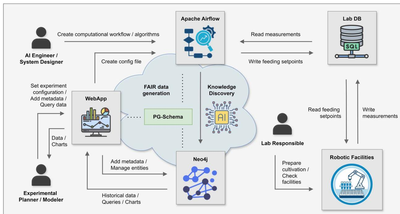
Fig. 3 Overall architecture. Apache Airflow interacts with the SQL database that coordinates laboratory devices, and stores data and metadata in Neo4j graph database with a property graph schema. A web application is included to configure the experiment, manage nodes metadata and query the knowledge graph.
