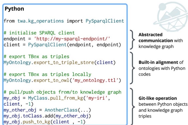
Fig. 2 Example usage of the twa Python package for interacting with knowledge graphs at both the TBox and ABox levels. The left panel shows concise Python operations for initialising a SPARQL client, exporting class hierarchies as triples to both remote endpoints and local files, and synchronising Python object states with their RDF representations in the knowledge graph. The annotations on the right side clarify the conceptual benefits.
