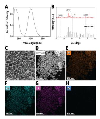
Fig. 8 (A) The in-situ obtained UV-Vis absorption and PL spectra, (B) XRD pattern, (C) TEM image, and (D–H) HAADF-STEM image of the highest-performing  $Cs_3Cu_2I_5$  NCs synthesized by the SDFL using the El decision-making policy.
