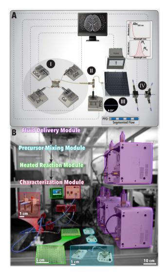
Fig. 2 The developed SDFL for autonomous manufacturing and optimal synthetic route discovery of  $Cs_3Cu_2l_5$  NCs utilizing a one-pot heat-up synthesis approach in the presence of a halide additive, Znl<sub>2</sub>: (A) schematic illustration of the (I) fluid delivery, (II) precursor mixing, (III) flow reactor, and (IV) *in situ* characterization modules of the SDFL. (B) A color-coded image of the SDFL.
