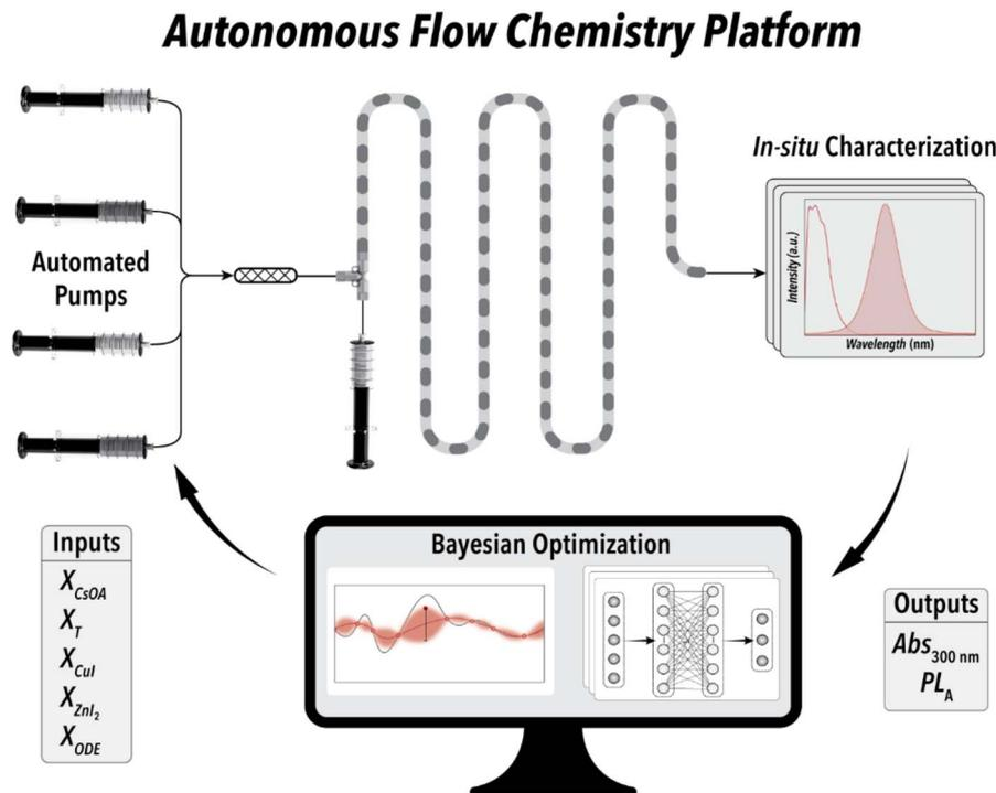
Fig. 1 Illustration of an autonomous fluidic lab for closed-loop synthesis science studies of Cu-based MHP NCs.
