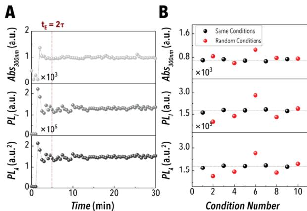
Fig. 3 Evaluation of the SDFL's hardware robustness for prolonged operation and reproducible in-flow synthesis of Cu-based MHP NCs: (A) time-resolved progression of Abs<sub>300 nm</sub>, PL<sub>I</sub>, and PL<sub>A</sub> under a specific synthesis condition over 30 min. (B) Reproducibility studies of the SDFL hardware through a cross-contamination study.
