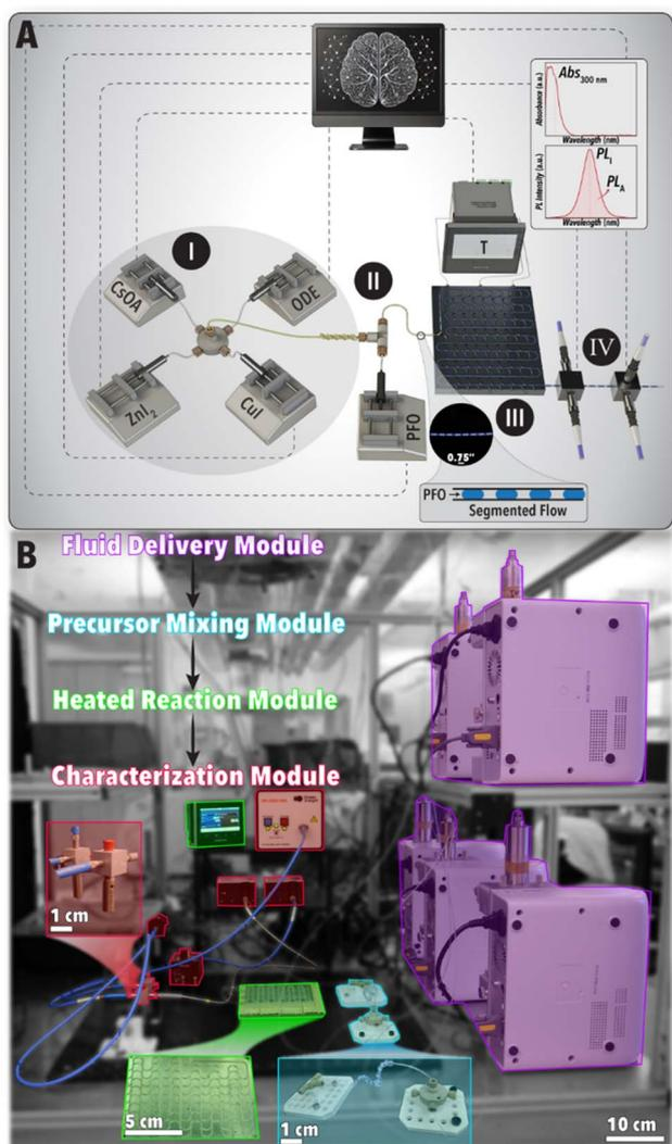
Fig. 2 The developed SDFL for autonomous manufacturing and optimal synthetic route discovery of  $\text{Cs}_3\text{Cu}_2\text{I}_5$  NCs utilizing a one-pot heat-up synthesis approach in the presence of a halide additive,  $\text{ZnI}_2$ : (A) schematic illustration of the (I) fluid delivery, (II) precursor mixing, (III) flow reactor, and (IV) *in situ* characterization modules of the SDFL. (B) A color-coded image of the SDFL.
