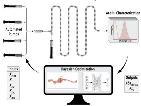
Fig. 1 Illustration of an autonomous fluidic lab for closed-loop synthesis science studies of Cu-based MHP NCs.
