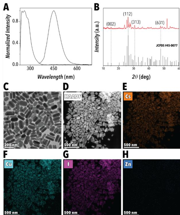
Fig. 8 (A) The in-situ obtained UV-Vis absorption and PL spectra, (B) XRD pattern, (C) TEM image, and (D–H) HAADF-STEM image of the highest-performing  $\text{Cs}_3\text{Cu}_2\text{I}_5$  NCs synthesized by the SDFL using the EI decision-making policy.
