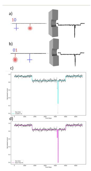
Fig. 4 (a) Schematic view of a two-bit barcode in the 10-configuration translocating a nanopore. The 4-arm star represents the 0 bit, the 12arm star represents the 1 bit. (b) Schematic view of a two-bit barcode in the 01-configuration translocating a nanopore. (c) CUSUM+ fit on DNA Nanostructures Barcodes event. (d) Nano Trees fit on DNA Nanostructures Barcodes event
