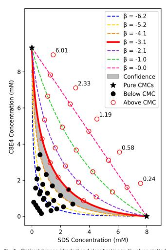
Fig. 6 Optimal  $\beta$  range (shaded) and classification truth values plotted over the regular solution theory  $\beta$  curves for the SDS-C<sub>8</sub>E<sub>4</sub> system, where the optimal  $\beta$  range represents the region that minimizes the number of misclassifications. The numbers in the figure are the actual ratios of surfactants used in the experiments.
