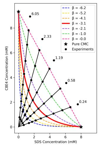
Fig. 1 Regular solution theory mixed CMC curves overlaid with five constant composition lines evenly spaced about the pink dashed ideal mixing line. Proposed experimental trials are mapped from the five constant composition lines, with additional points below and above the curves to sandwich the sampling space. The numbers in the figure indicate the ratio of the surfactants to use in each line.
