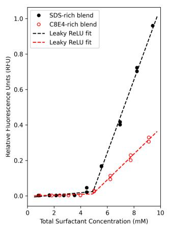
Fig. 3 Leaky ReLU regression upon the most SDS-rich blend and most C<sub>8</sub>E<sub>4</sub>-rich blend to judge the suitability of the fit and the resulting CMC value. For the SDS-rich blend, the SDS/C<sub>8</sub>E<sub>4</sub> ratio is 4.149. For the  $C_8E_4$ -rich blend, the ratio is 0.166
