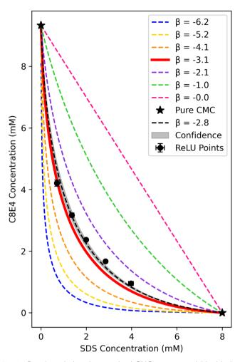
Fig. 4 Regular solution theory mixed CMC curves overlaid with the five ReLU-regressed CMC points and the resulting orthogonally regressed regular solution theory boundary with the quantified  $\beta$  interaction parameter and 95% confidence interval (shaded region).
