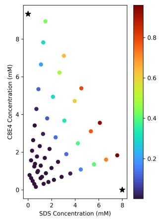
Fig. 2 2D visualization of the normalized fluorescence intensity as a function of the two surfactant concentrations for the SDS- $C_8E_4$  system, with an observable fluorescence jump (black to dark blue) marking the onset of micellization.
