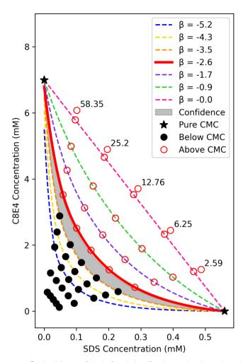
Fig. 7 Optimal  $\beta$  range (shaded) and classification truth values plotted over the regular solution theory  $\beta$  curves for the SDS-C<sub>8</sub>E<sub>4</sub> in 0.5 M NaCl system, where the optimal  $\beta$  range represents the region that minimizes the number of misclassifications. The numbers in the figure are the actual ratios of surfactants used in the experiments
