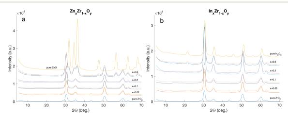
Fig. 8 Stacked pairs of XRD patterns of all materials retrieved from the four production campaigns of  $Zn_xZr_{1-x}O_y$  (a) and  $In_xZr_{1-x}O_y$  (b). The dashed lines represent the corresponding replication batches with the same nominal composition.
