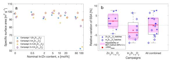
Fig. 7 (a) Individual BET-surfaces for all 28 batches issued from the four production campaigns represented by four different marker types. (b) Box plot of the relative batch-to-batch variation of specific surface area (SSA) for pairs with the same composition issued from separate production campaigns.
