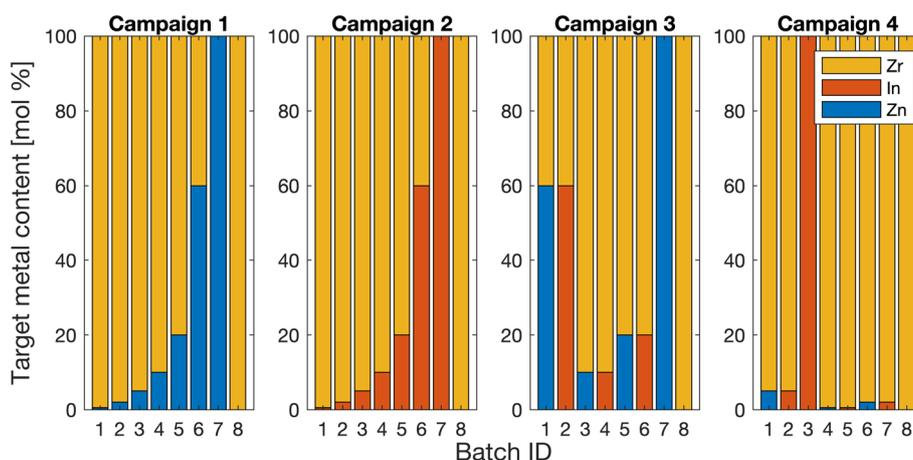
Fig. 2 Production campaigns 1 and 2 were run to synthesize Zn<sub>x</sub>Zr<sub>1-x</sub>O<sub>y</sub> and In<sub>x</sub>Zr<sub>1-x</sub>O<sub>y</sub>, with varying molar loadings of In on Zr and Zn on Zr, respectively. Therein, the use of Zn and In precursors was not alternated, ruling out any possible contamination. In contrast, campaigns 3 and 4 were designed to quantify batch-to-batch carryover.
