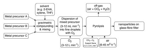
Fig. 1 Block flow diagram of steps performed during FSP synthesis. These must be performed in both manual and automatic modes.
