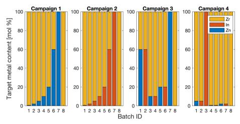
Fig. 2 Production campaigns 1 and 2 were run to synthesize  $Zn_xZr_{1-x}O_y$  and  $In_xZr_{1-x}O_y$ , with varying molar loadings of In on Zr and Zn on Zr, respectively. Therein, the use of Zn and In precursors was not alternated, ruling out any possible contamination. In contrast, campaigns 3 and 4 were designed to quantify batch-to-batch carryover.
