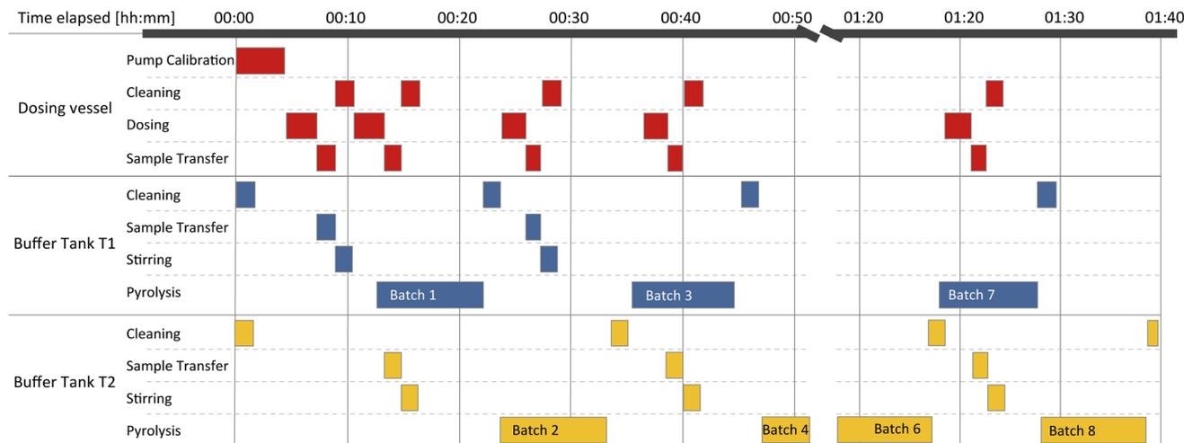
Fig. 10 Gantt chart of process steps during production campaign 4. The rate limitation of the overall production speed by the pyrolysis step is worth noting, which in turn cannot be shortened further, but is a given parameter. Shown here are the preparation of precursor mixtures and the pyrolysis of batches 1, 2, 3, and 8.
