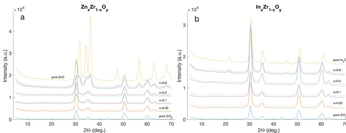
Fig. 8 Stacked pairs of XRD patterns of all materials retrieved from the four production campaigns of  $\text{Zn}_x\text{Zr}_{1-x}\text{O}_y$  (a) and  $\text{In}_x\text{Zr}_{1-x}\text{O}_y$  (b). The dashed lines represent the corresponding replication batches with the same nominal composition.
