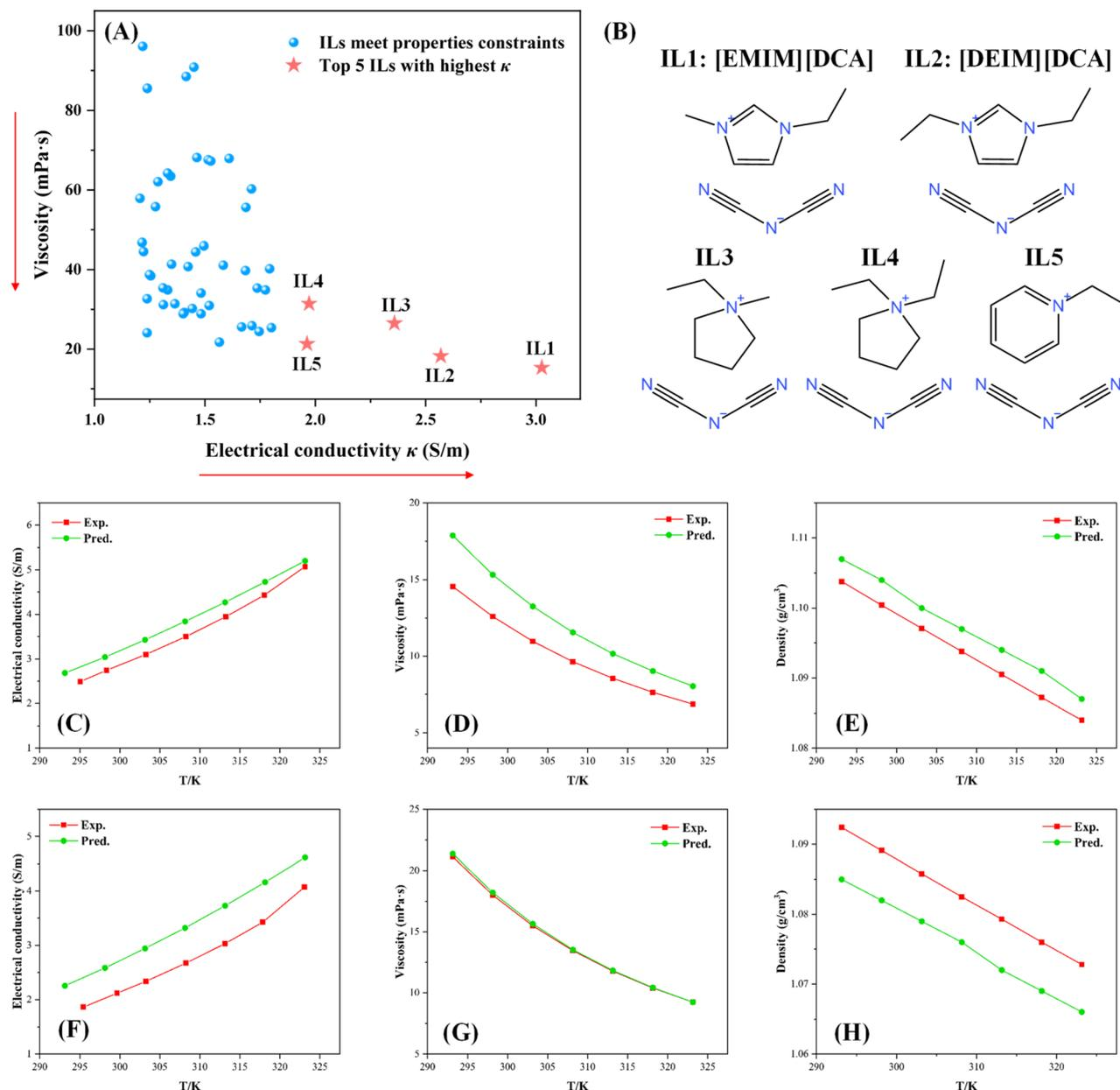
Fig. 8 High-throughput screening results and experimental validation for ILs as electrolytes. (A) Viscosity and electrical conductivity of 50 candidate ILs. The top five ILs with the highest electrical conductivity are highlighted with red stars. (B) Structures of the five screened ILs with the highest electrical conductivity. (C–E) Electrical conductivity, viscosity and density of [EMIM][DCA]. (F–H) Electrical conductivity, viscosity and density of [DEIM][DCA].
