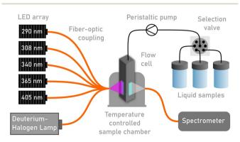
Fig. 1 Schematic of the photoswitch characteristation platform.
