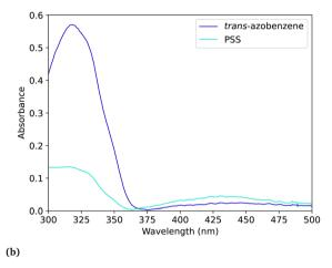
Fig. 4 (a) Reaction scheme for the azobenzene photoisomerisation. (b) UV-Vis spectra of the trans-azobenzene and the photostationary state (PSS) with cis-azobenzene following irradiation at 340 nm.
