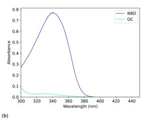
Fig. 2 (a) Reaction scheme for the norbornadiene-quadricyclane (NBD-QC) photoswitch pair. (b) Corresponding UV-Vis spectra of the photoswitch pair.
