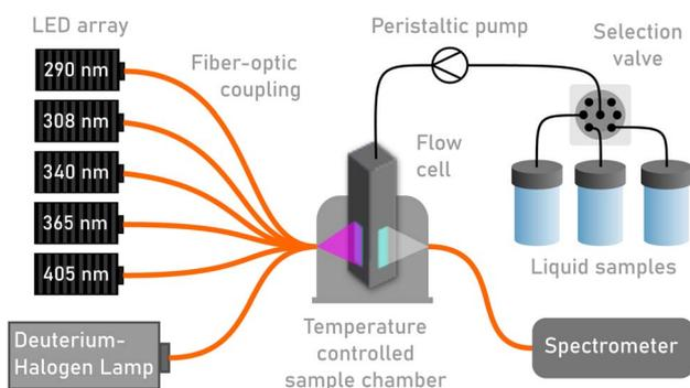
Fig. 1 Schematic of the photoswitch characterisation platform.
