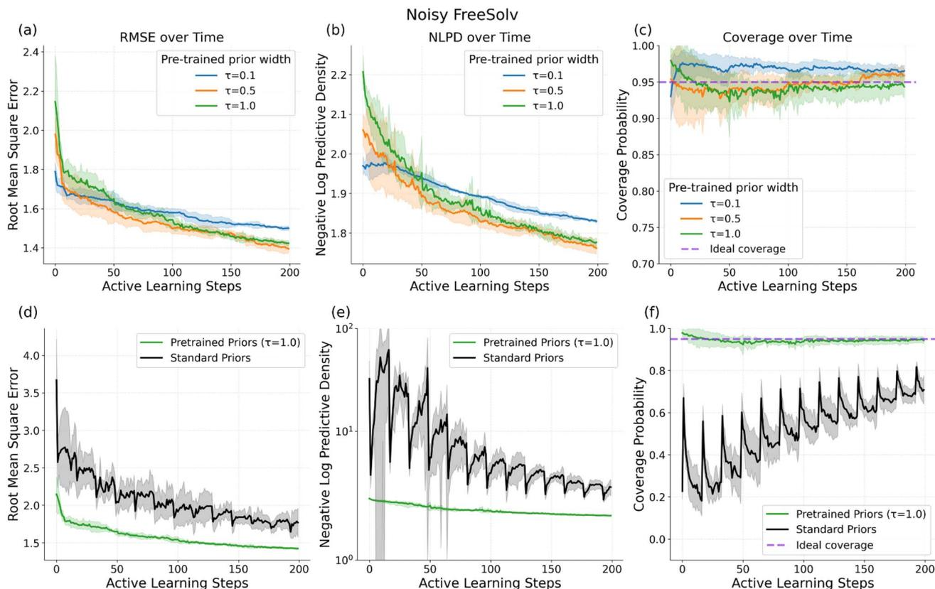
Fig. 7 Transfer learning with pre-trained PBNNs applied to noisy FreeSolv dataset. (a) RMSE, NLPD, and coverage probability for different prior widths ( $\tau$ ). (b) Comparing the performance of pre-trained priors ( $\tau = 1.0$ ) against standard priors. Shaded areas represent a standard deviation across five different random seeds.
