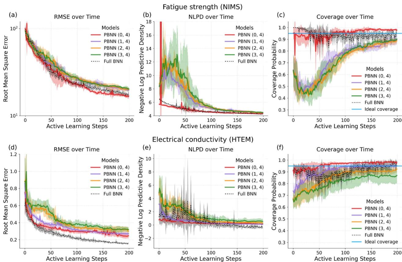
Fig. 5 Comparison of Partially Bayesian Neural Networks (PBNNs) and fully Bayesian neural network (full BNN) on materials property prediction tasks. (a–c) Fatigue strength prediction (NIMS database) and (d–f) electrical conductivity prediction (HTEM database). Each PBNN configuration PBNN ( $i$ , 4) has two probabilistic layers: one at position  $i$  (counting from 0) and one at the output. Shaded areas represent a standard deviation across five different random seeds.
